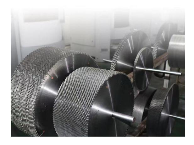
SAW BODY CAN USE 75CR1 STEEL AND JAPAN SKS51 STEEL. TIPS WITH IMPORTED KIND WITH LONGER CUTTING LIFE. DIAMETER RANGE: 80-2200 MM CAN BE PROVIDED.
